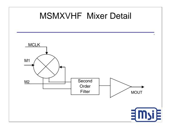
The mixer of the MSMXVHF provides a continuous time second order lowpass filter set at approximately 1 MHz. Since the maximum switched capacitor filter center/corner frequency is up to 1 MHz, this filter reduces any local oscillator clock (MCLK) feedthrough.
