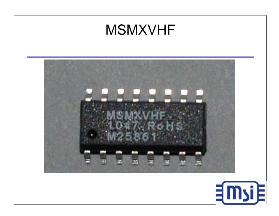
Here is a photograph of the MSMXVHF. The device is available in a SOIC-16 150 mil narrow package (39 mm square excluding leads) and a VQFN-28 4x4mm (16 mm square) in the future. Although these parts are packaged in Lead-free RoHS plastic and leadframes, we can supply in more traditional Tin/Lead lead finish.
