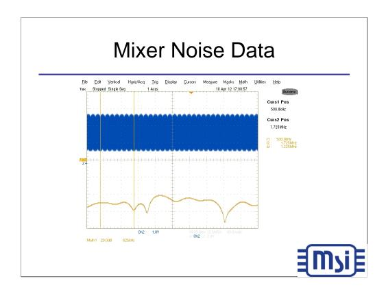
The noise data is taken with a 15 MHz LO and the mixer clock inputs grounded. The top trace of the scope display shows the mixer clock input in the time domain. The bottom trace of the display shows the output of the mixer in the frequency domain. The mixer output has been observed as low as -80 dB.
