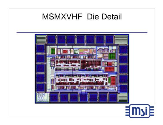
This is a plot of the device layout of the MSMXVHF. The design is in 0.35um double-Polysilicon, double-metal CMOS. The die is small enough to easily fit into a 28 leadless VQFN 4x4mm package.
