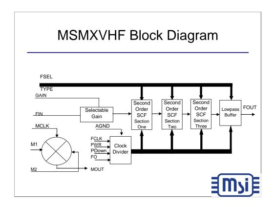
This is the block diagram of the MSMXVHF. The mixed-signal mixer is independent of the filter section. Two synchronized clocks of different frequencies can be used to separate the mixer local oscillator from the filter clock, which sets the filter center frequency (for bandpass) or corner frequency (for lowpass).
