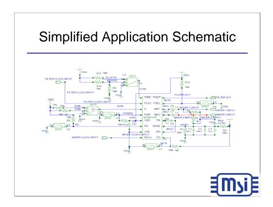
The simplified schematic shows the connections of the MSMXVHF with signals and clocks. FOUT is the filtered output from the mixer/filter combination. The switches for filter type, lowpass or bandpass, power, powerdown, and clock-to-corner ratio are CMOS levels.
