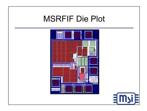
This plot is of the MSRFIF, showing the charge pump and filtering capacitors. The device is integrated in a 0.6 um double-polysilicon, double metal CMOS process.
