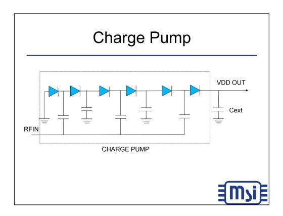
Here is an simplified block diagram of a charge pump. Using diodes and capacitors, received AC signals are rectified and filtered onto capacitors. The switching action of the transistor allows charge to be built up on the capacitor up to the voltage limit of the clamp diodes (4V).
