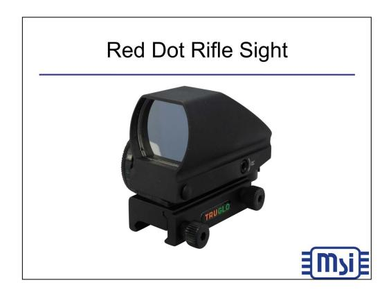
This photograph is of the Truglo Red Dot Rifle Sight. This sight uses a CR2032 battery with a choice of either red or green dot and dot intensity. The CR2032 battery has the shortest life with the brighter red LED selected. With green LED selected the device draws 5 mA at its brightest setting.
