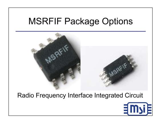
The MSRFIF is available in both a SOIC-8 package, 150 mils wide and a TSSOP-8 package 173 mils wide. The chips are almost always smaller than an Antenna or Piezoelectric transducer.
