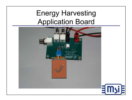
This photograph is of the MSRFIF evaluation board with Mide'Technology Center's Volture V25W piezoelectric wafer attached. The charge pump in the MSRFIF takes the input from the piezoelectric wafer and outputs DC to the binding posts. The MSRFIF is also capable of amplitude shift keying demodulation. If the vibration of the piezo device can be modulated, data can be demodulated by the MSRFIF.
