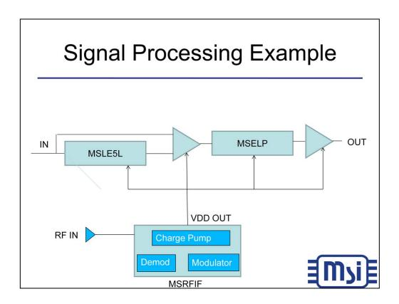
Here is an example of a potential application. Using our standard products and our MSRFIF , a bandpass filter can be created. These building blocks can be integrated into a single integrated circuit. The MSLE5L 5<sup>th</sup> order Elliptic lowpass filter with an op amp from the MSELP will produce a highpass filter. The MSELP will provide a lowpass filter. The MSELP contains an RC operating mode which can clock both filters.
