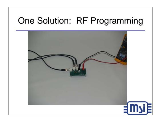
This photograph is of the MSRFIF evaluation board. The MSRFIF is an integrated circuit with a high frequency charge pump, modulator and demodulator and power detect output. No power supply is needed. The received signal powers up the device and supplies up to 50 uA at 2.4V to other circuits. The device includes an AM and Bi-phase PSK demodulator. Low power microcontrollers can be powered by the MSRFIF.
