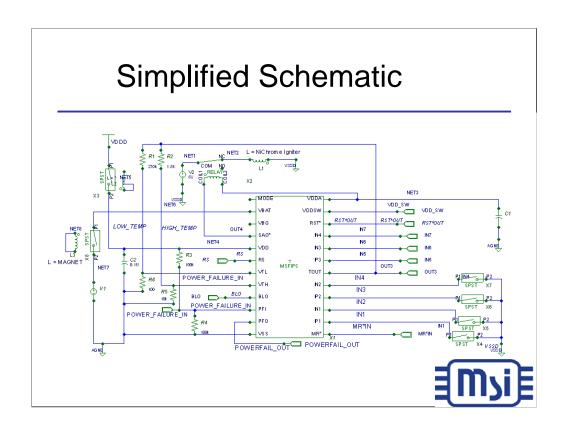
The simplified schematic shows the connections of the MSFIPS with batteries and the relay for the igniter. Most applications, the SAO\* output is not tied to a relay, but, is tied to a microcontroller to wipe memory.
